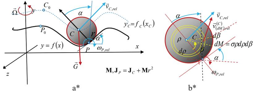
FIGURE 17. Geometric parameters of the rolling of heavy rigid disks on a rotating curvilinear trace in a vertical plane around a vertical axis
