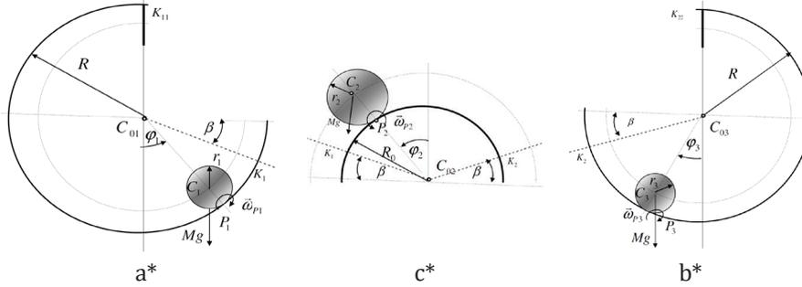
FIGURE 13. Decomposition of the rolling ball dynamics along the curvilinear line rolling trace consisting of three circle arches
