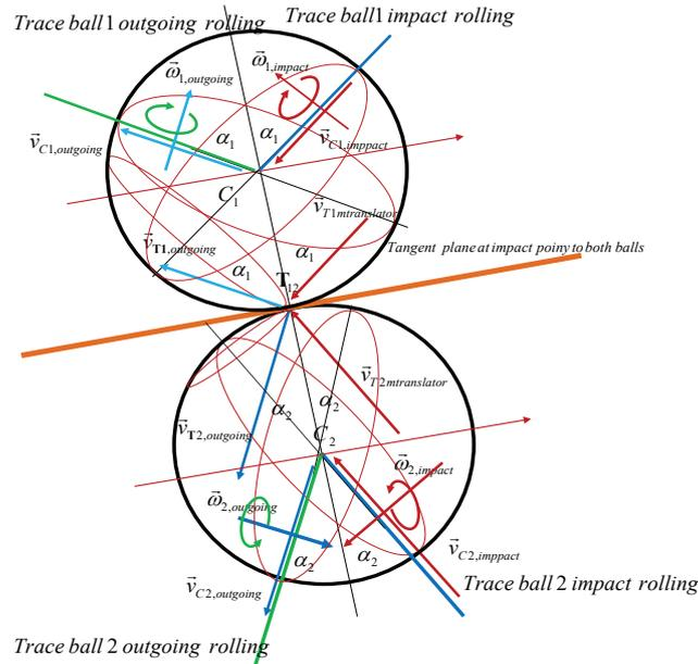
FIGURE 26. Collision of two rolling balls and the plan of incoming and outgoing angular velocities of the rolling balls with their rolling paths before and after an oblique collision
