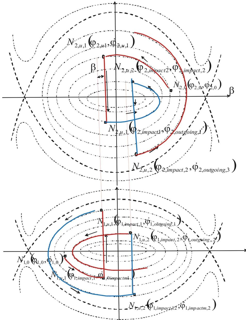
FIGURE 11. Phase trajectory portraits of vibro-impact dynamics of rolling balls along a curvilinear circular line in a vertical plane with two first successive collisions: (upper) for the second rolling ball and (lower) for the first rolling ball
