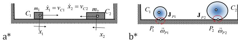
FIGURE 8. Models of the two simplest dynamics of material bodies, each with one degree of freedom of movement: a\* translatory dynamics of a rigid body and b\* rolling without slipping of a rigid body (with a form of a homogeneous disk, a homogeneous sphere or homogeneous with one axis and one plane of symmetry).
