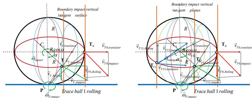
FIGURE 23. Plan of the velocity of impact of a point on a large circle of a sphere, which rolls along a straight line in a horizontal plane
