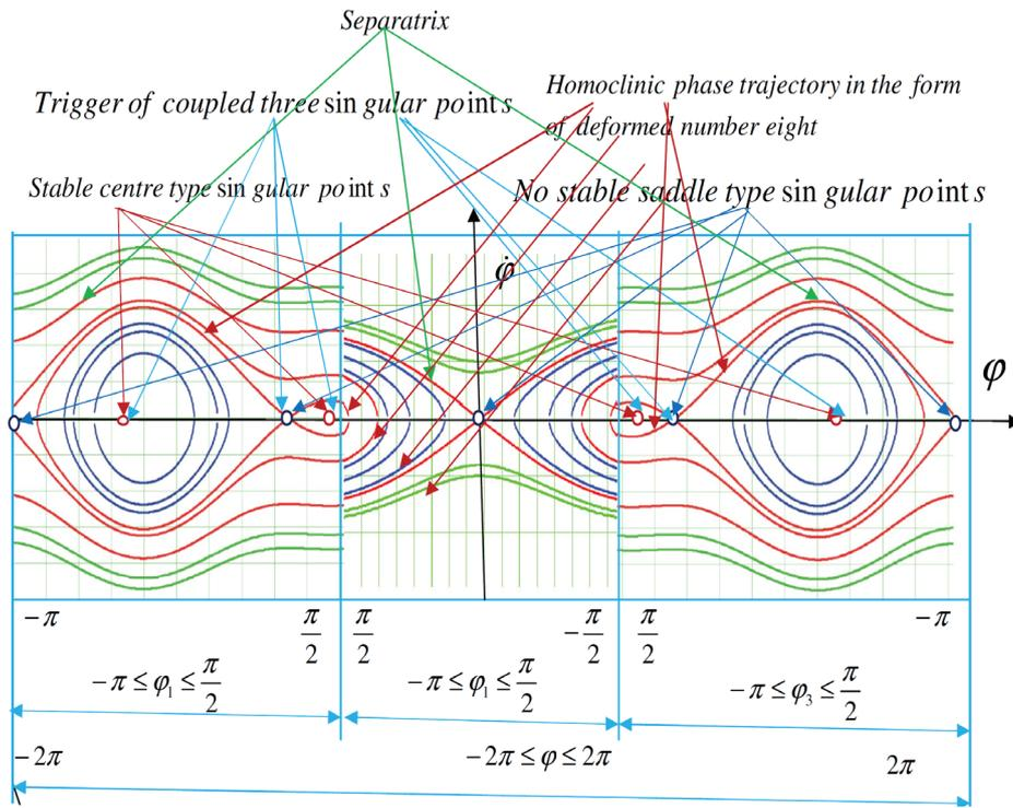
FIGURE 19. One combination of many possible parts of phase trajectory portraits finalized into a complex phase trajectory portrait of a dynamics of a relative rolling heavy thin disk along a rotating curvilinear trace around a vertical axis of its symmetry at a constant angular velocity, with the notation of the corresponding set of singular points, and two triggers of coupled singular points and homoclinic trajectory orbits in a form of two deformed figure eight shapes
