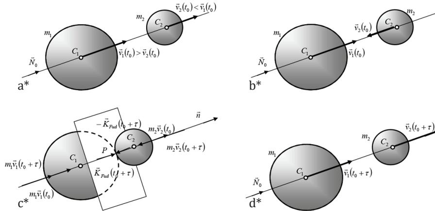
FIGURE 3. Central collision between two bodies, with mass  $m_1$  and  $m_2$  in translatory motion (a\* and b\*) and with translatory pre-impact velocities  $\vec{v}_1(t_0)$  and  $\vec{v}_2(t_0)$  (c\*) and with outgoing post-impact velocities  $\vec{v}_1(t_0 + \tau)$  and  $\vec{v}_2(t_0 + \tau)$  (c\* and d\*).
