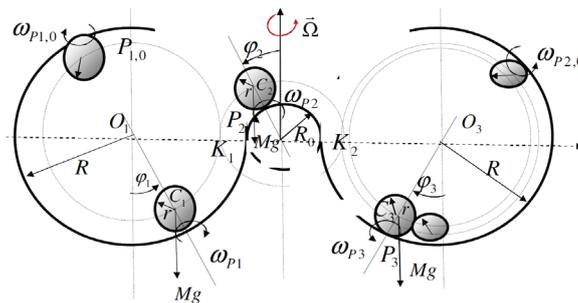
FIGURE 18. Vibro-impact system, containing two generalized rolling pendulums each in the form of a thin heavy disk, which are in rolling motions, without slipping, along a rotating curvilinear line trace with the constant angular velocity  $\Omega$  around the vertical axis of a curvilinear line axial symmetry
