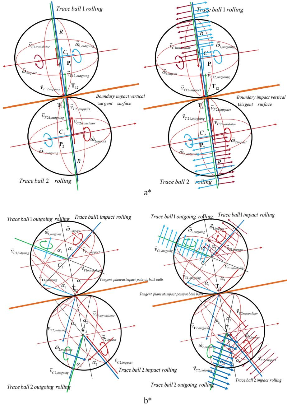
FIGURE 27. Partial analogies between the central and oblique collisions of two rolling balls: the opening of the traces of ball rolling in the oblique (skew) collision (b \*) with respect to the central collision of the balls (a \*).
