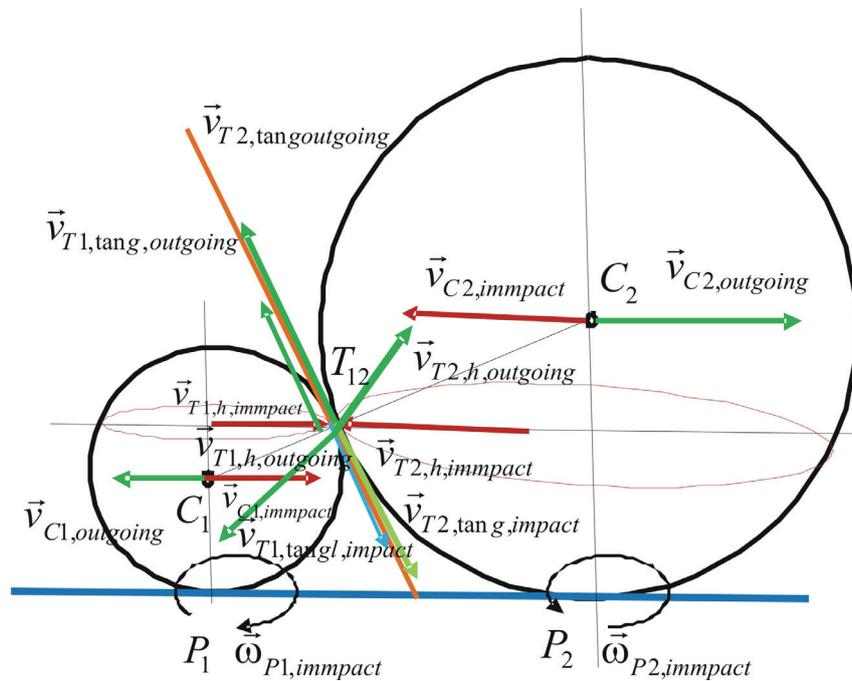
FIGURE 7. Plans of the component impact and outgoing velocities at the point of central collision of two rolling heavy balls with different radiuses
