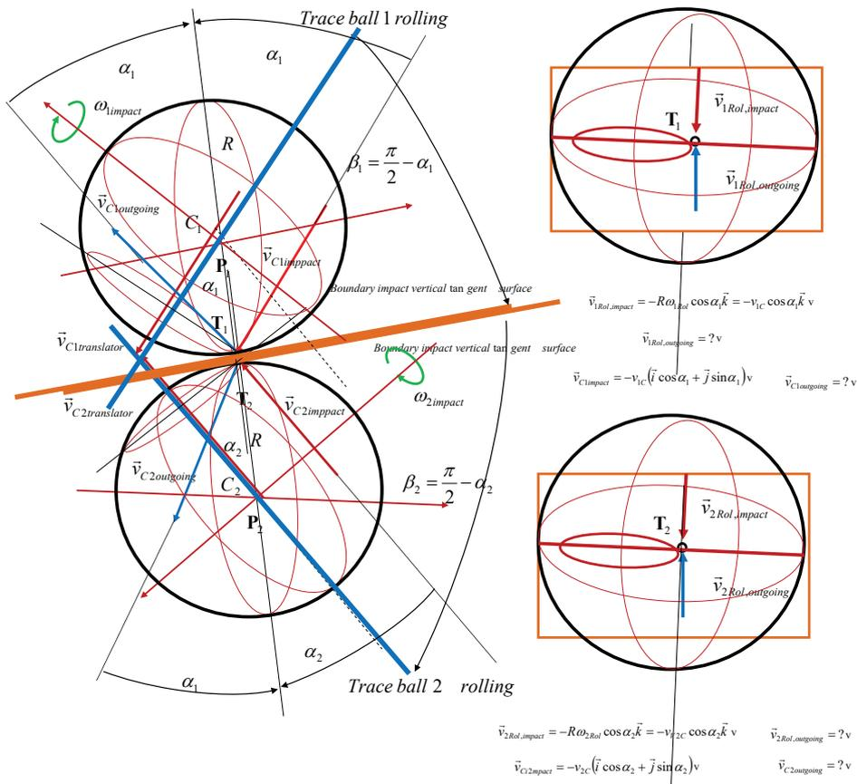
FIGURE 25. A system of two equal billiards balls that roll on rolling tracks in an oblique (skew) collision configuration. The plan of the incoming and outgoing velocities of the collision points of each of the two balls at their oblique collision
