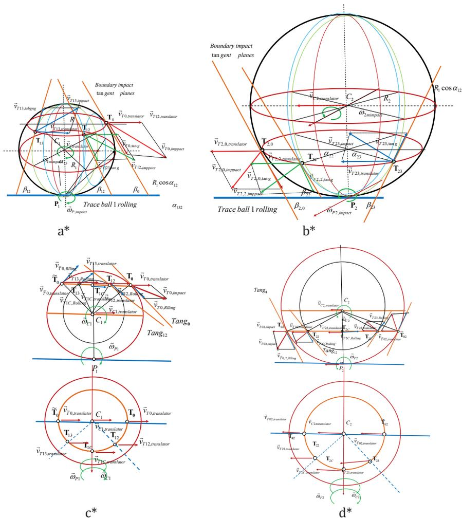
FIGURE 5. Plans of the impact velocities of possible points of collision of two rolling heavy balls with different radii: a\* and c\* for the first rolling smaller ball and b\* and d\* for the second biggest rolling ball.
