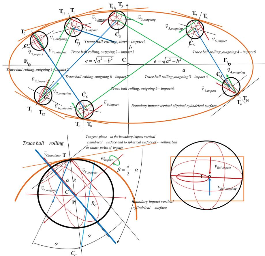
FIGURE 22. Line-trace of the rolling motion of the ball along the horizontal plane of the elliptical billiards with the plan of horizontal components of the incoming impact velocities and the outgoing velocities of the contact point after the impact of the ball into a contour elliptical cylindrical surface with vertical derivatives (up); Detail of the plan of the velocity of one ball in the configuration of the skew impact (down)
