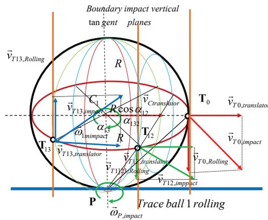
FIGURE 4. Plan of component impact velocities of impact points of a ball for the different types of collisions of two equal rolling balls
