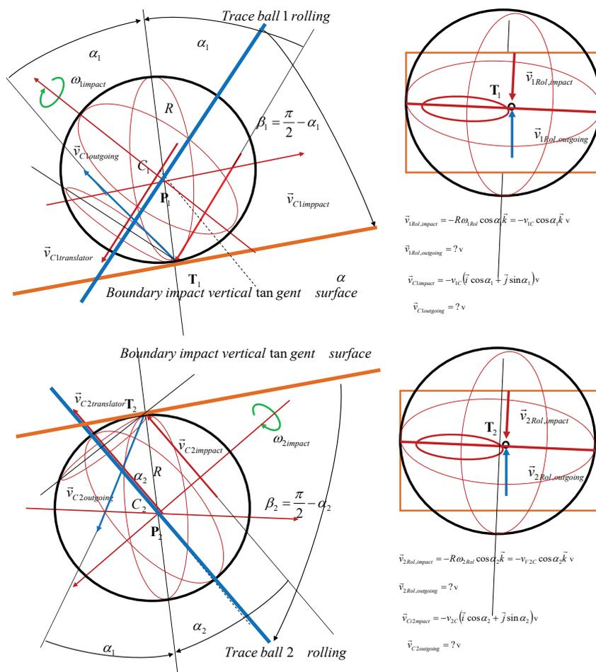
FIGURE 24. Decomposed system of two equal billiard balls in configuration of an oblique (skew) collision. Plan of the incoming and outgoing velocities of the collision contact points of each of the two balls at their oblique collision.
