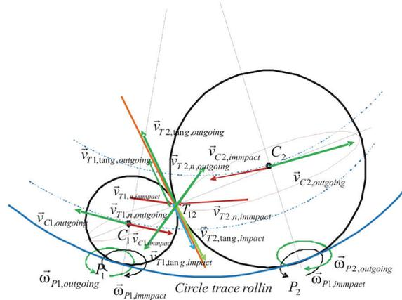
FIGURE 10. Plan of angular velocities and component velocities in pre- and post-collision of two rolling heavy balls along a circular trace in a vertical plane
