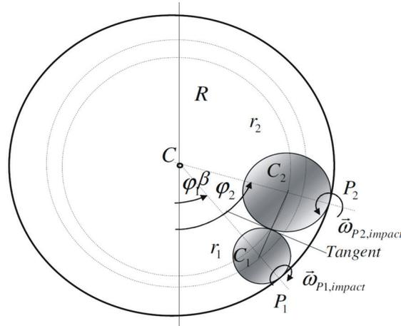
FIGURE 9. Mechanical system of collision of two heavy rolling balls along a circular trace in a vertical plane
