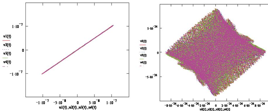
FIGURE 4. a. Full synchronization (angles  $\pi/6$  and  $\pi/4$ ). b. Full asynchronization for (angles  $\pi/2$  and  $\pi/2$ ) of all four ZP 1 molecules from representative part of the mZP oscillatory net.
