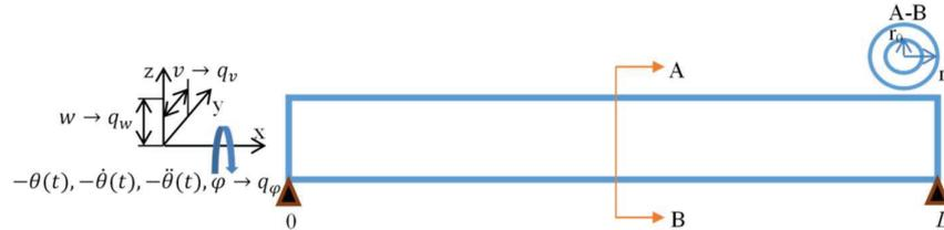
FIGURE 1. The configuration of the spinning shaft, with the coupled generalized coordinates of deformations ( $v, w, \varphi$ ), their associated modal generalized coordinates ( $q_v, q_w, q_\varphi$ ), and the associated direction of the angular rigid body coordinate ( $\theta$ ), velocity ( $\dot{\theta}$ ), and acceleration ( $\ddot{\theta}$ ).
