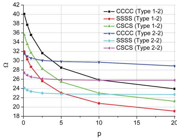
FIGURE 9. Variation of the fundamental frequency parameter  $\Omega_L^{(1)} = \lambda_1 a^2 \sqrt{\rho_c / E_c} / h$  of the spherical shells with increasing gradient index  $p$
