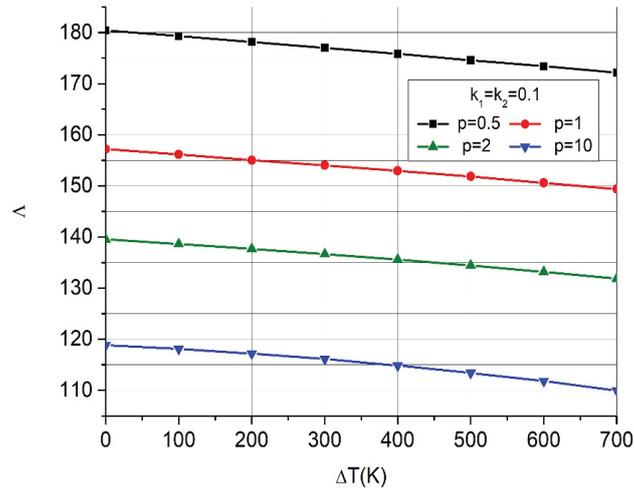
FIGURE 14. Effect of volume fraction index  $p$  on the natural frequencies parameters of the clamped FG spherical panels with clamped square cutout subjected to nonlinear temperature rise
