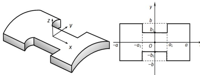
FIGURE 6. FGM shell panel with rectangular cuts
