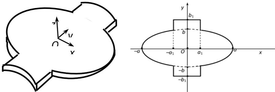
FIGURE 2. FGM shallow shell with complex shape and its planform
