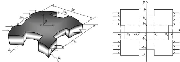
FIGURE 15. FGM shallow shell with complex planform and its planform
