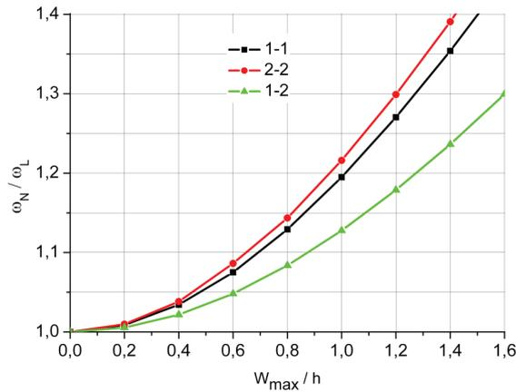
FIGURE 11. Backbone curves for clamped cylindrical shells (1-8-1,  $p=0.5$ ,  $Al / Al_2O_3$ )
