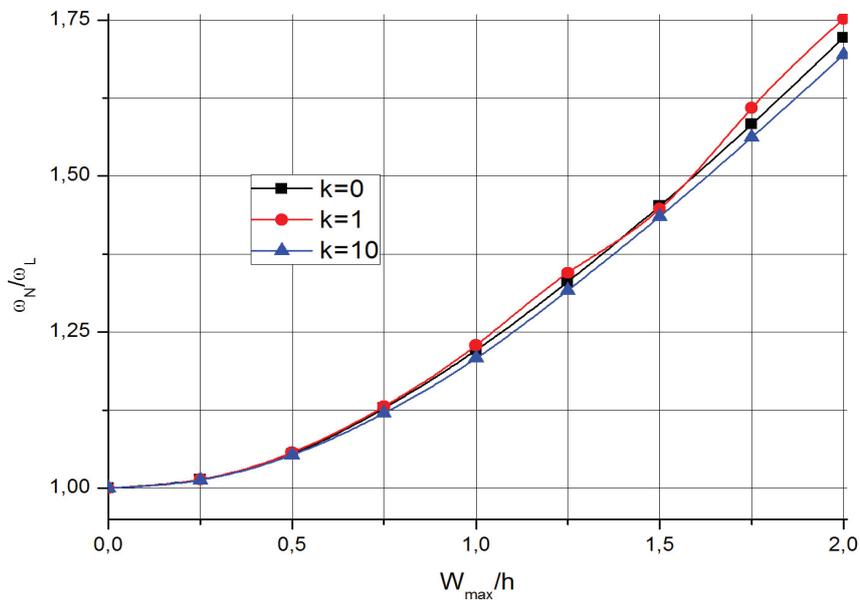
FIGURE 4. Backbone curves for clamped spherical shells made of FGMs  $Al/ZrO_2$
