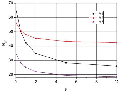
FIGURE 16. Effect of gradient index on critical load of the clamped (CL) shells for different types of material
