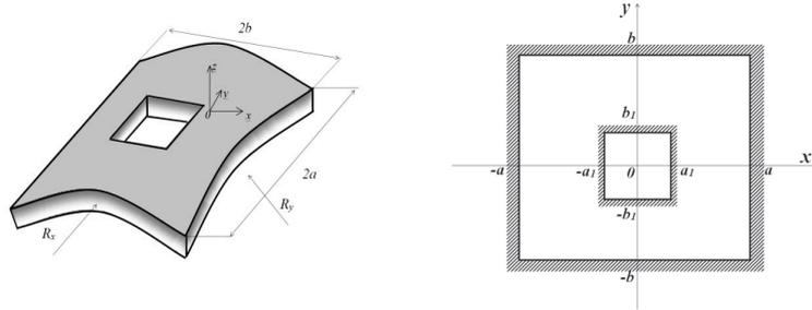
FIGURE 13. FGM shallow shell with inner cutout and its planform
