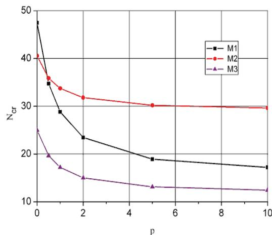
FIGURE 17. Effect of gradient index on critical load of the simply supported (SS) shells for different types of material
