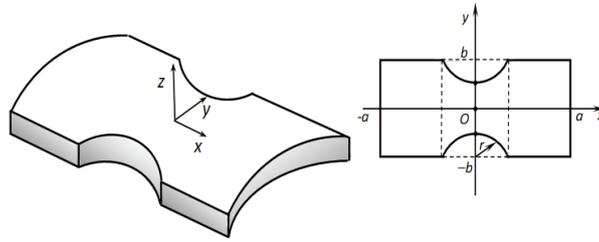
FIGURE 7. FGM shell panel with circular cuts
