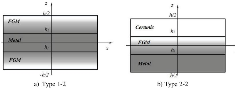
FIGURE 8. Schemes of lamination of the layers
