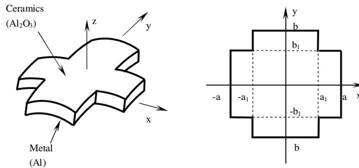
FIGURE 5. FGM shallow shell with cutout and its planform
