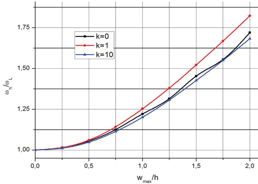
FIGURE 3. Backbone curves for clamped spherical shells made of FGMs  $Al/Al_2O_3$
