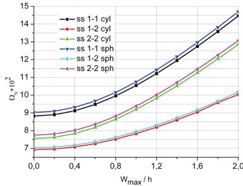
FIGURE 12. Backbone curves for simply-supported (SS) spherical (sph) and cylindrical (cyl) shells with lamination scheme (1-8-1,  $p=0.5$ ,  $Al / Al_2O_3$ )
