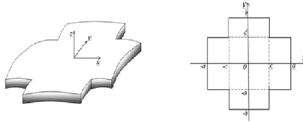
FIGURE 10. Shape of the plan of the laminated FGM shallow shell
