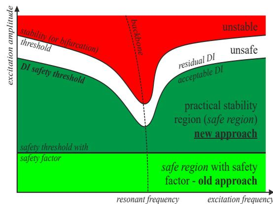
FIGURE 11. Schematic safety chart for a softening system subjected to harmonic excitation [5].
