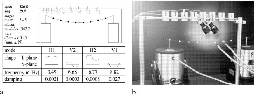
FIGURE 6. Experimental cable-mass system. (a) Mechanical model with parameters and dynamical characteristics; (b) Hanged nylon wire carrying eight small concentrated masses, with shakers and two movable optical cameras.
