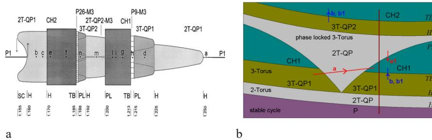
FIGURE 7. Quasiperiodic scenario to chaos. (a) Experimental bifurcation diagram, (b) canonical two-parameter bifurcation chart for 3-Torus breakdown, with partially similar qualitative scenario along the vertical brown line (H: Hopf, PL: phase-locking, TB: torus breakdown, SC: saddle cycle; periodic (Pm-M3), quasiperiodic (nT-QPm-Mk) and chaotic (CH1, CH2) attractors) [4].
