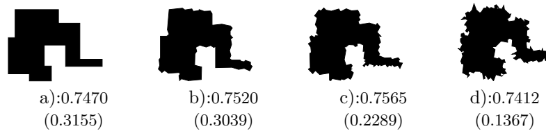
FIGURE 4. \mathbf{C}(S) circularities of shapes with added noise are given immediately below the shapes. The corresponding \mathbf{C}_{st}(S) circularities are in brackets.
