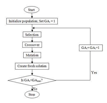
Figure 1: Flow chart for genetic algorithm
