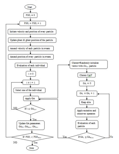
Figure 2: Flow chart for genetic algorithm
