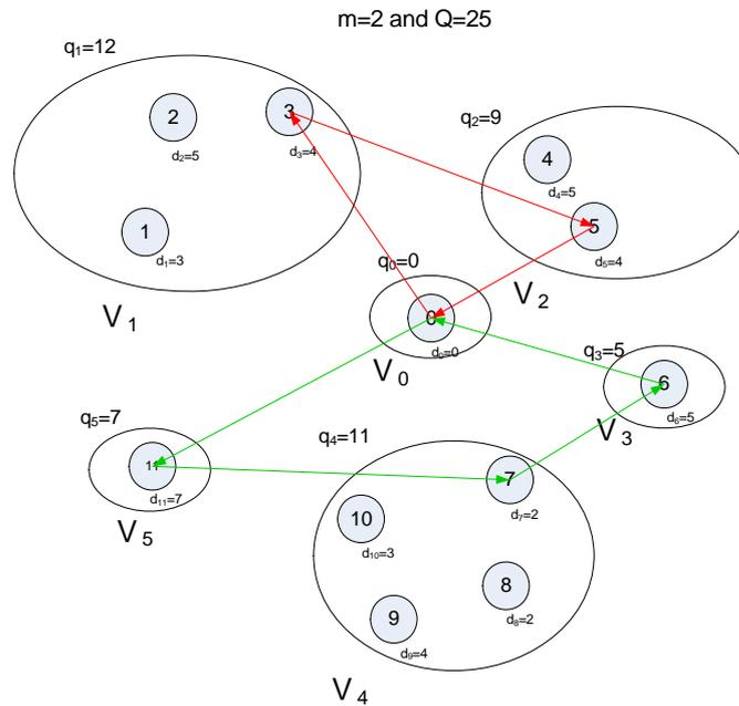
**Figure 1:** A feasible solution to the Generalized Vehicle Routing Problem
