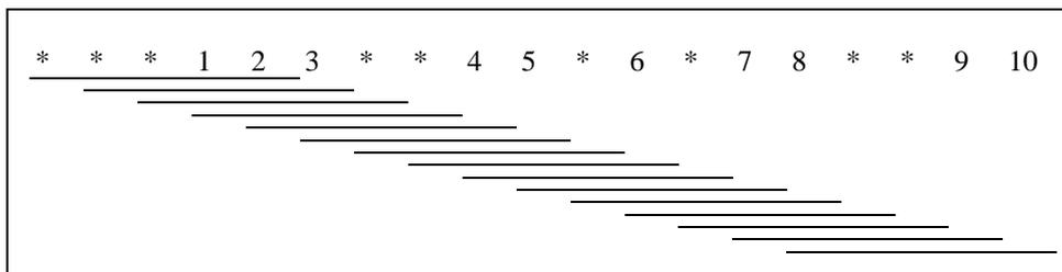
Figure 3:  $C(5,19; F)$  system. Alternative representation of minimal cuts with the insertions of 9 artificial “broken-down” components (\*)
