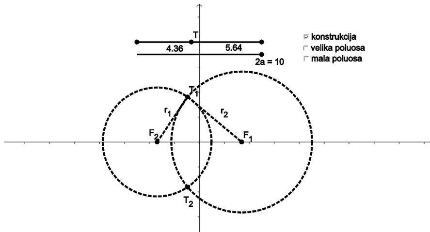
Figure 1. A detail of a GeoGebra dynamic worksheet representing the pins-and-string method for the ellipse construction
