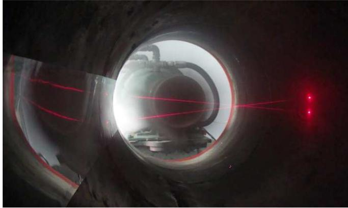
FIGURE 2. Laser Doppler anemometer measurements in a diffuser
