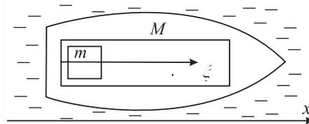
FIGURE 15. Body with a movable internal mass in a resistive medium
