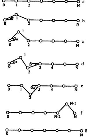
FIGURE 5. Wave-like motion with three moving links
