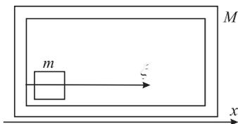
FIGURE 14. Body with a movable internal mass on a plane
