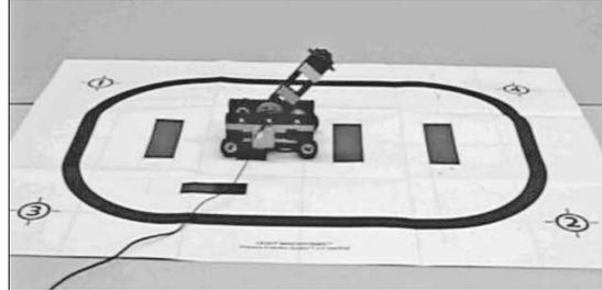
FIGURE 17. Cart with inverted pendulum
