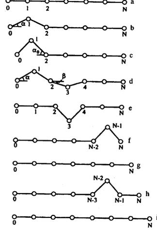
FIGURE 6. Wave-like motion with four moving links
