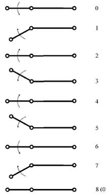
FIGURE 3. Phases of periodical motion of a two-link system
