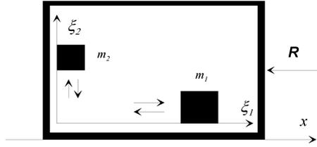
FIGURE 16. Body with two internal masses
