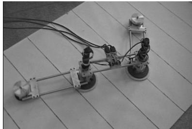
FIGURE 4. Experimental model of a three-link system
