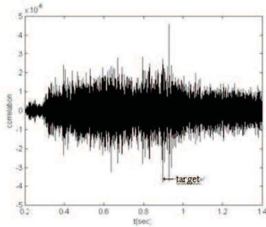
Figure 18: Signal that include the reverberation and the target at 600 m is processed with modified AGC and cross correlation.
