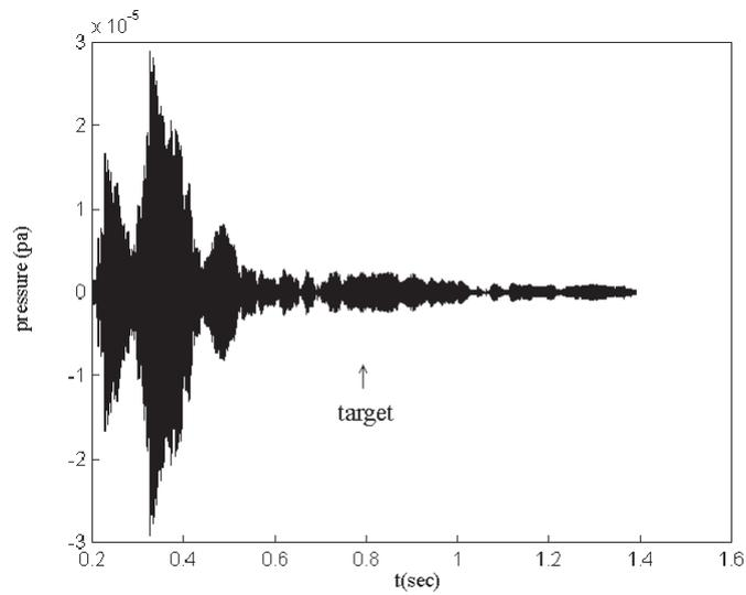
Figure 8: Signals of the reverberation and the target. The target is 600 m away from the source.
