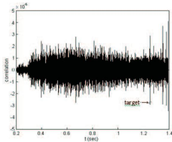
Figure 20: Signal that include the reverberation and the target at 900 m is processed with modified AGC and cross correlation.
