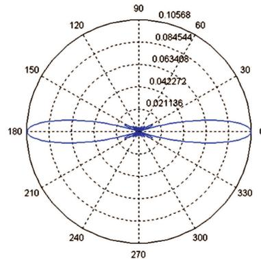
Figure 3: Beam-pattern of a spherical steel ball for  $ka = 877$ .
