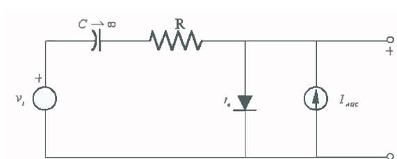
Figure 5: The circuit of a simple AGC
