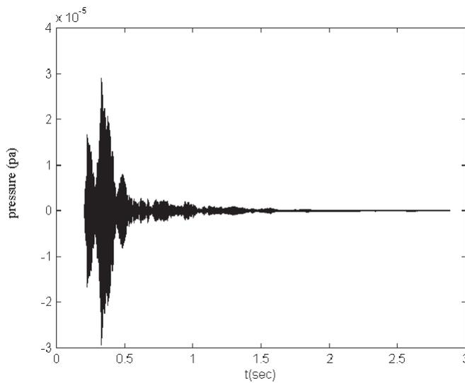
Figure 7: Signal of reverberation which is simulated by the model of image source with a CW transmission.
