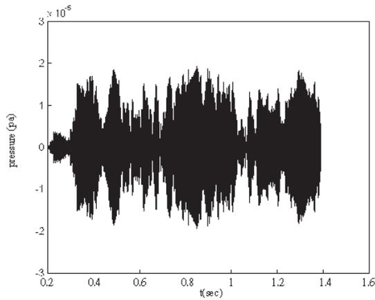
Figure 12: Signals that include the reverberation and the target at 600 m are processed with AGC.
