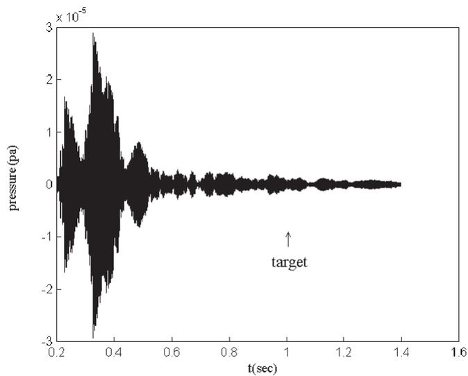
Figure 9: Signals of the reverberation and the target. The target is 750 m away from the source.
