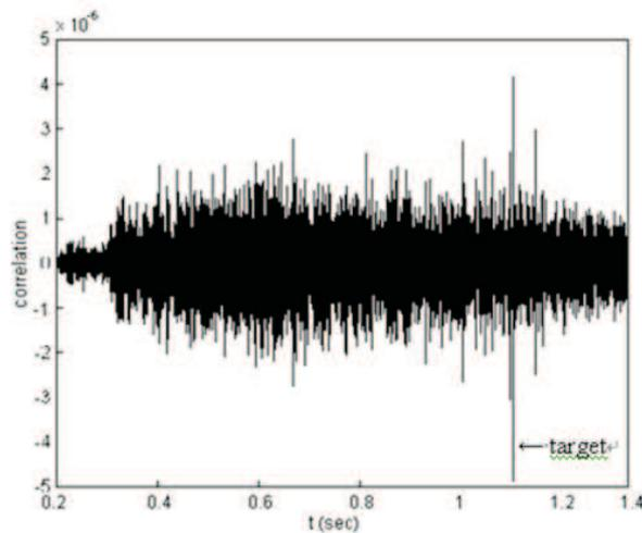
Figure 19: Signal that include the reverberation and the target at 750 m is processed with modified AGC and cross correlation.
