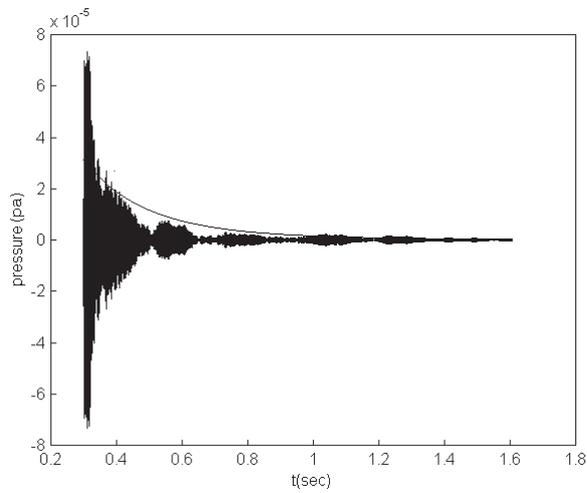
Figure 16: Sound pressure of the reverberation is shown in a CW source, where the control line is transformed from the curve of the sound energy.
