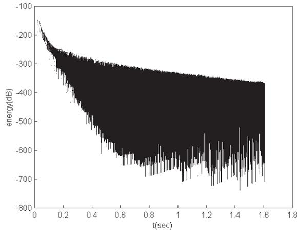
Figure 15: Energy of the reverberation with a pulse source.
