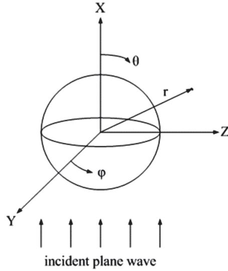
Figure 2: Plane harmonic compressional wave incident to a spherical ball.
