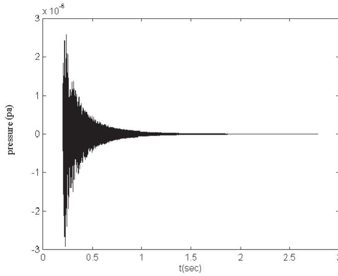
Figure 6: Signal of reverberation which is simulated by the model of image source with a pulse transmission.
