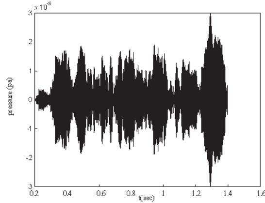
Figure 14: Signals that include the reverberation and the target at 900 m are processed with AGC.
