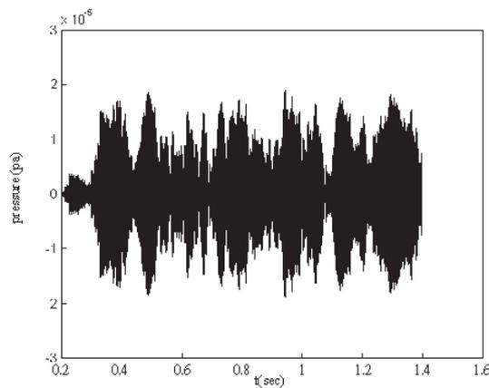
Figure 13: Signals that include the reverberation and the target at 750 m are processed with AGC.
