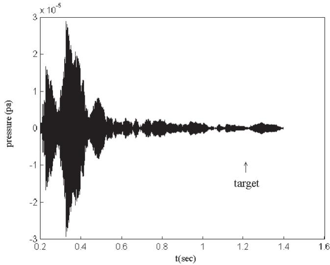
Figure 10: Signals of the reverberation and the target. The target is 900 m away from the source.
