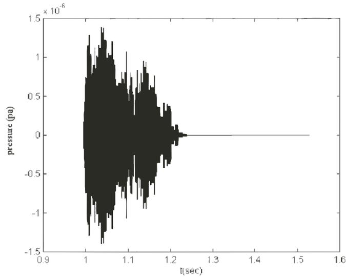
Figure 4: Signal of the target echo for the CW point source. The target is 750 m away from the source.
