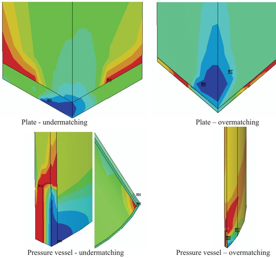
Figure 6: Final stage in increasing load: plastic zone reaches the interface
