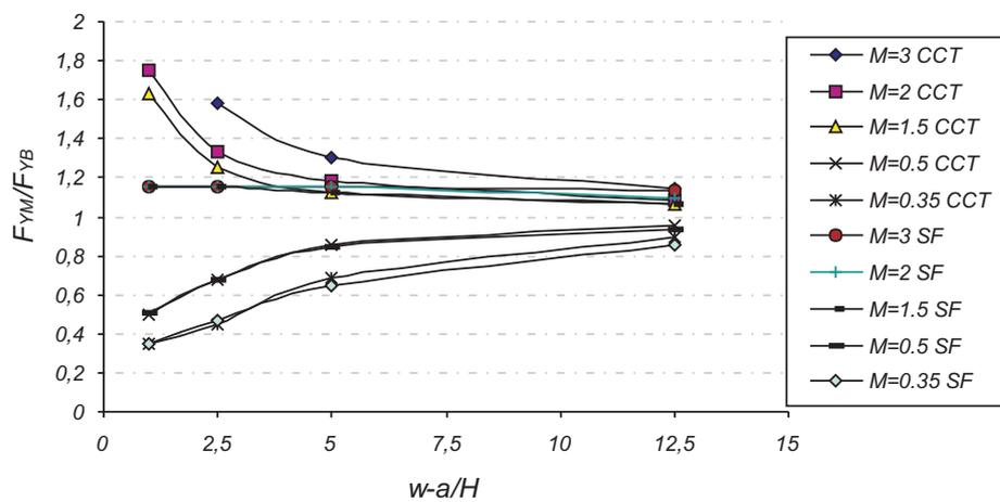
Figure 9: Limit load for different matching of CCT plate in plane strain and plate with surface crack for  $a/W = 0.5$
