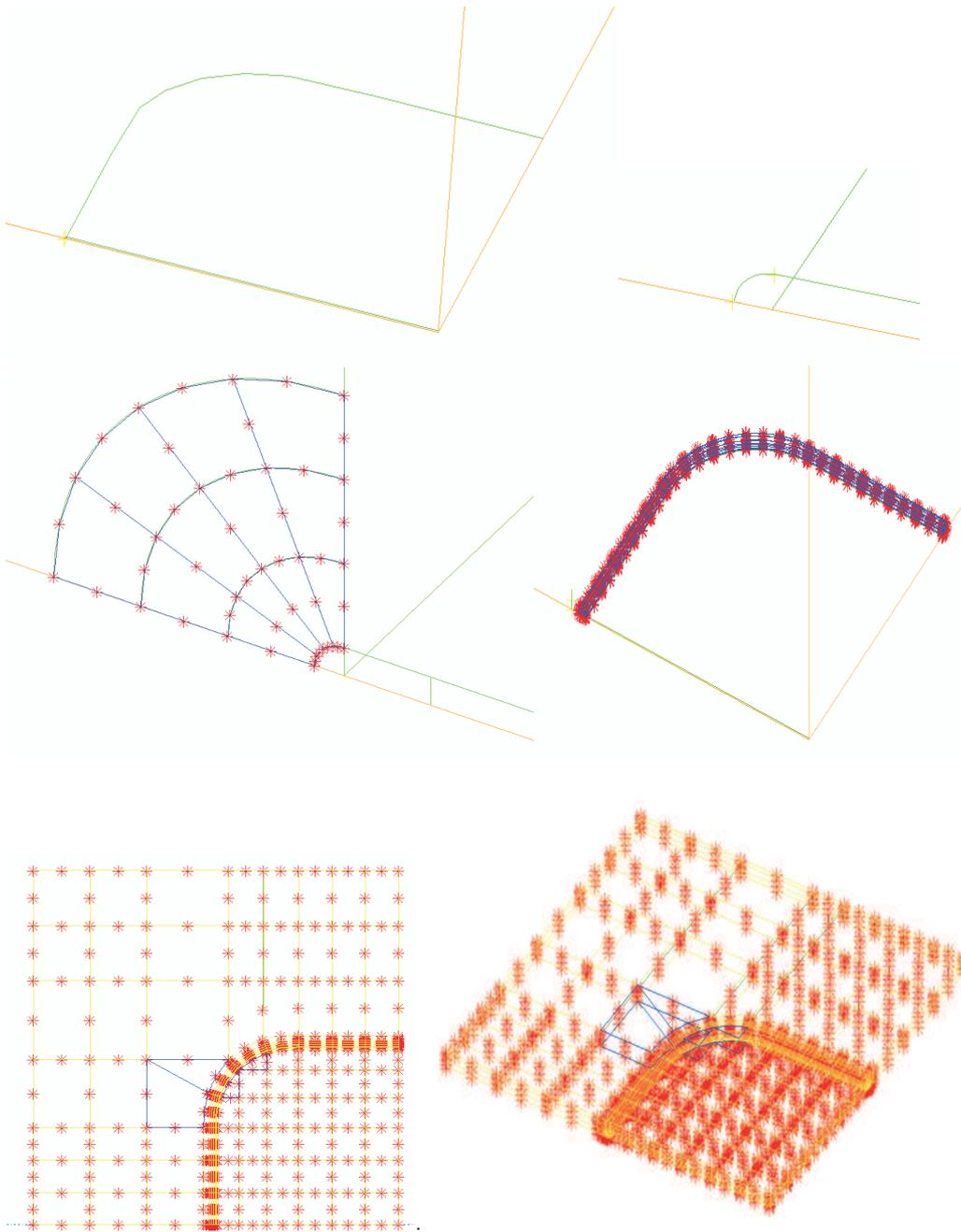
Figure 4: Mapping contour for surface crack in plate
