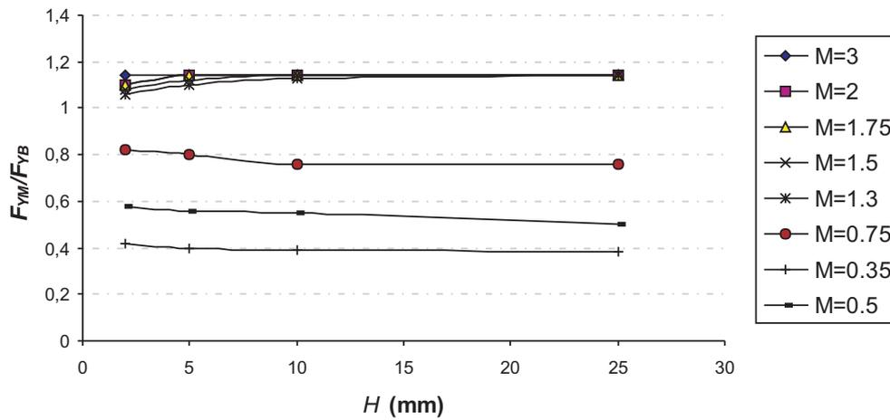
Figure 8: Limit load for different mismatch factor M for pressure vessel for  $t/a = 0.5$
