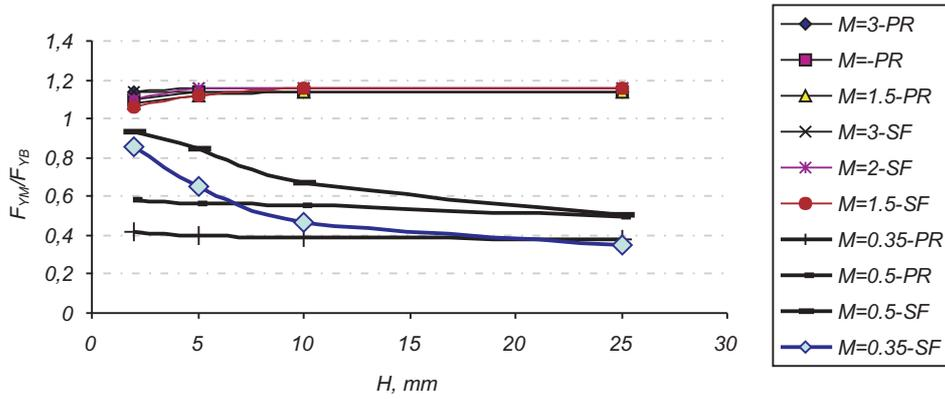
Figure 10: Limit load for different matching of pressure vessel for  $t/a = 0.5$ , and plate with surface crack
