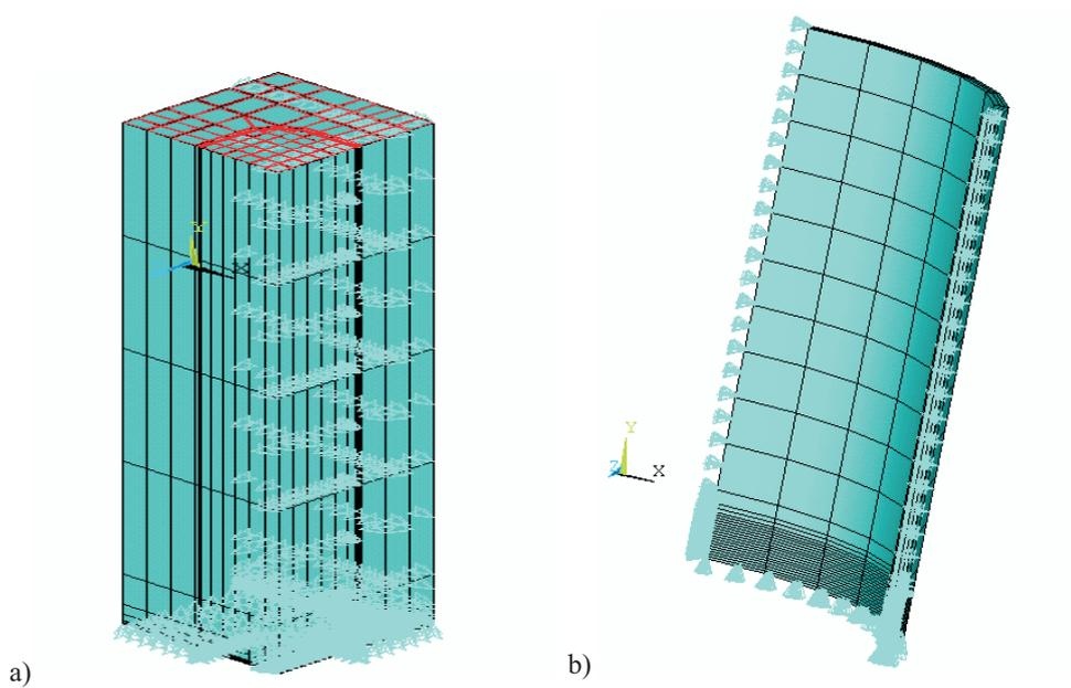
Figure 5: Finite element mesh for plate with surface crack (a) and pressure vessel (b)
