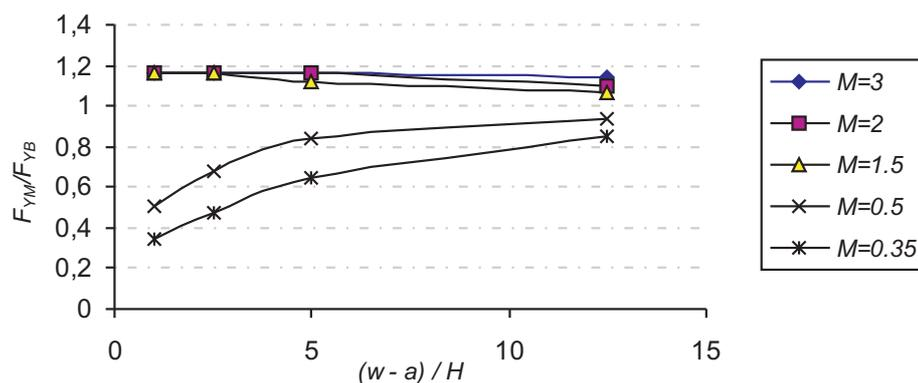
Figure 7: Limit load for different mismatch factor  $M$  of plate with surface crack for  $a/w=0.5$
