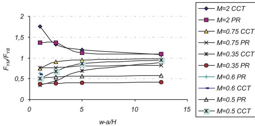
Figure 11: Limit load for different matching of CCT plate in plane strain for  $a/W = 0.5$  (2D) and pressure vessel (3D)
