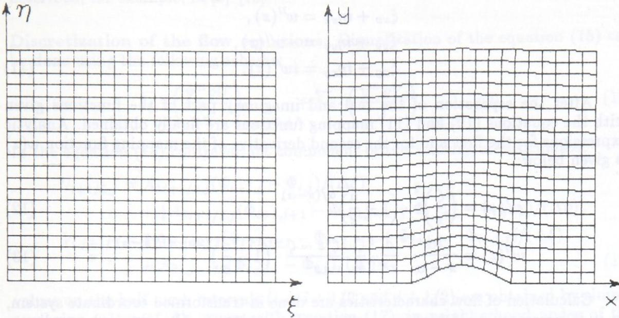
Figure 1: Calculation field in computational and physical plane
