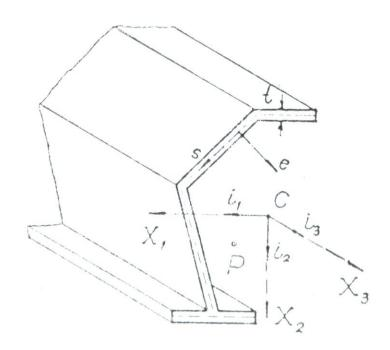
The position vector of an arbitrary point of the underformed memebr can be written for a fixed rectangular cartesain system  $x_i$  (i = 1,2,3) using the summation convention, in form
