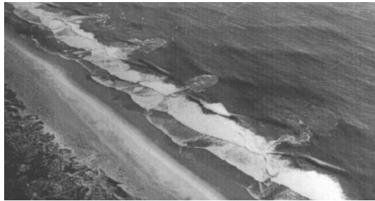
FIGURE 3. Rip currents periodic pattern [85]. Clearly visible are the necks and heads. The wide head of the currents indicates the merge of eddy couples.
