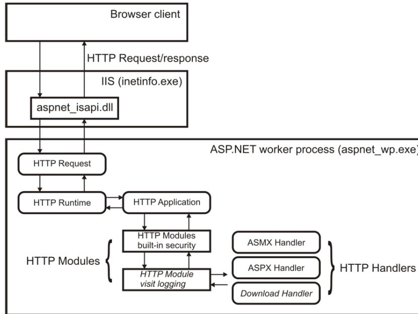
Figure 4: Overview of the extensions to the ASP.NET HTTP pipeline
