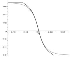
The first picture represents the graph of the exact solution and the approximate solution constructed by the proposed procedure upon the interval  $[d-2c_l\varepsilon,d+2c_r\varepsilon]$ , which includes interior layer. Quite modest values  $\varepsilon=10^{-2}$  and n=3 are chosen in purpose to distinguish the exact solution from the approximate one.
