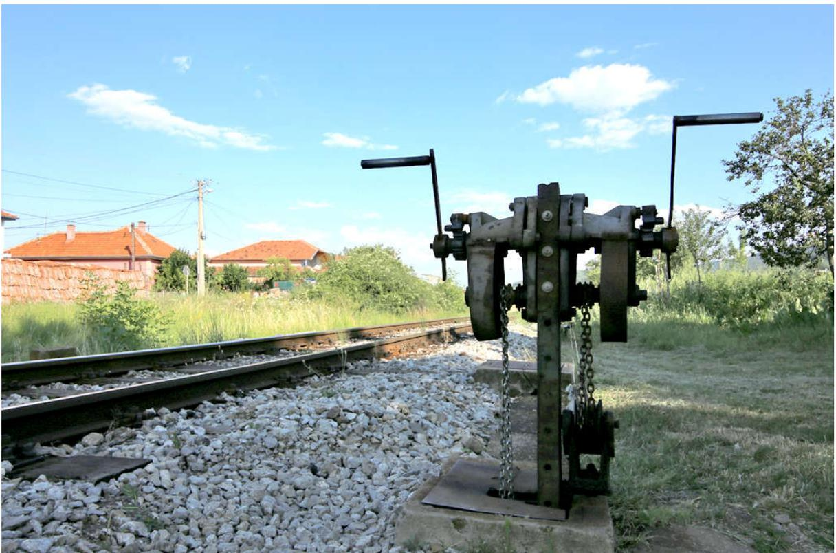
Figure 10. Winches for remote lowering and lifting barriers at the level crossings in Srećkovac, July 15, 2020 (Photo: Z. Cvetković)
