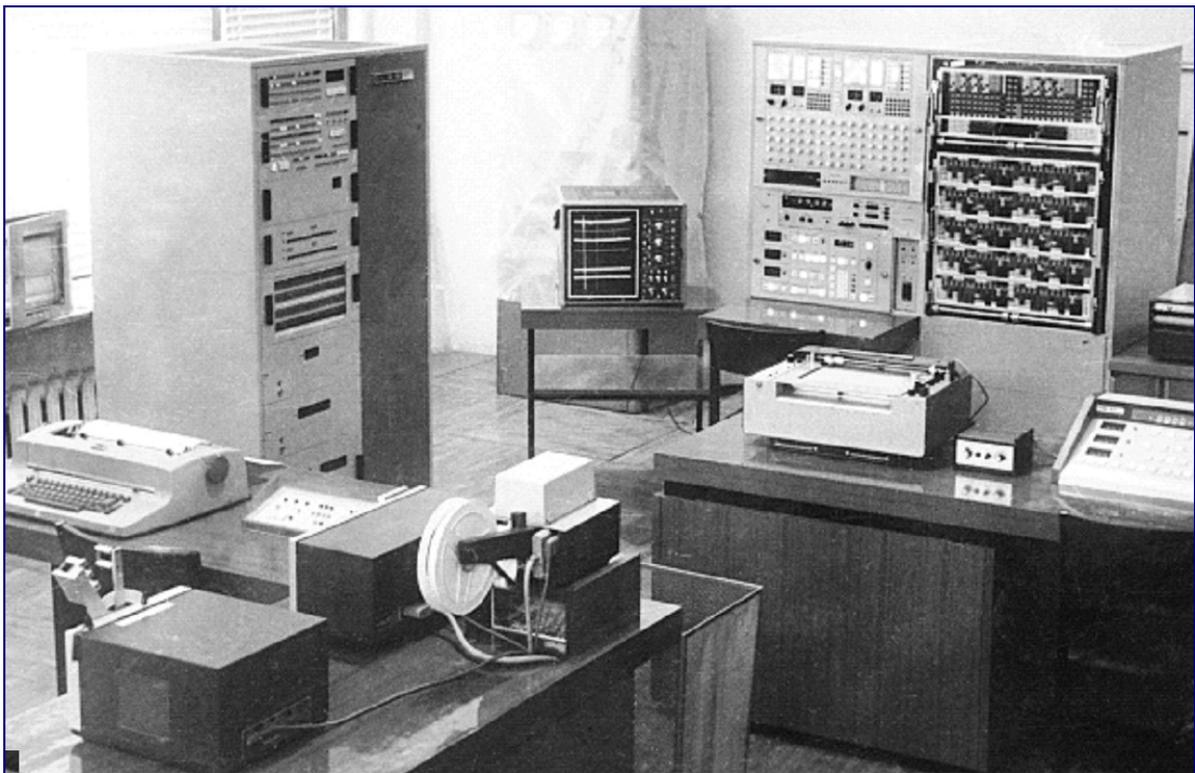
Figure 6. Hybrid system HRS 100
