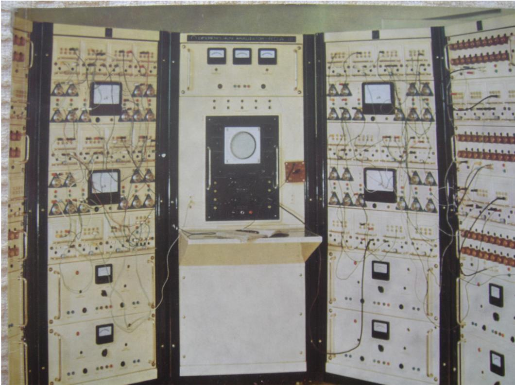
Figure 2. Repetitive Differential Analyzer
