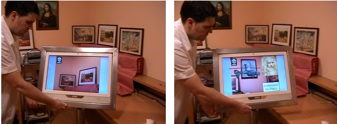
Figure 5 AR application example before (left) and after (right) detection of the marker
