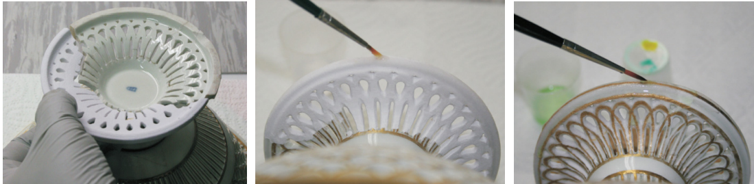
Picture 4: Supplementation of the bowl (less damaged) with 3D printed fragments (National Museum of Slovenia).
