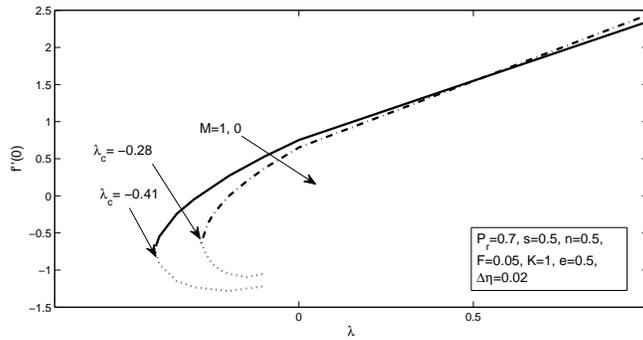
FIGURE 4. skin friction coefficient with  $M$
