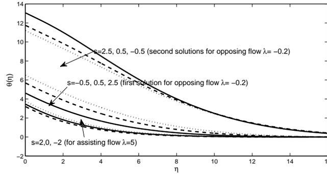
FIGURE 15. Temperature profiles for different  $s$
