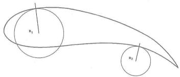
Where  $K_1 = \frac{1}{R_1}$ ,  $K_2 = \frac{1}{R_2}$  are curvatures of the wing surfaces, (values  $\epsilon_1, \epsilon_2$  dependent on  $K_1$  and  $K_2$ .
