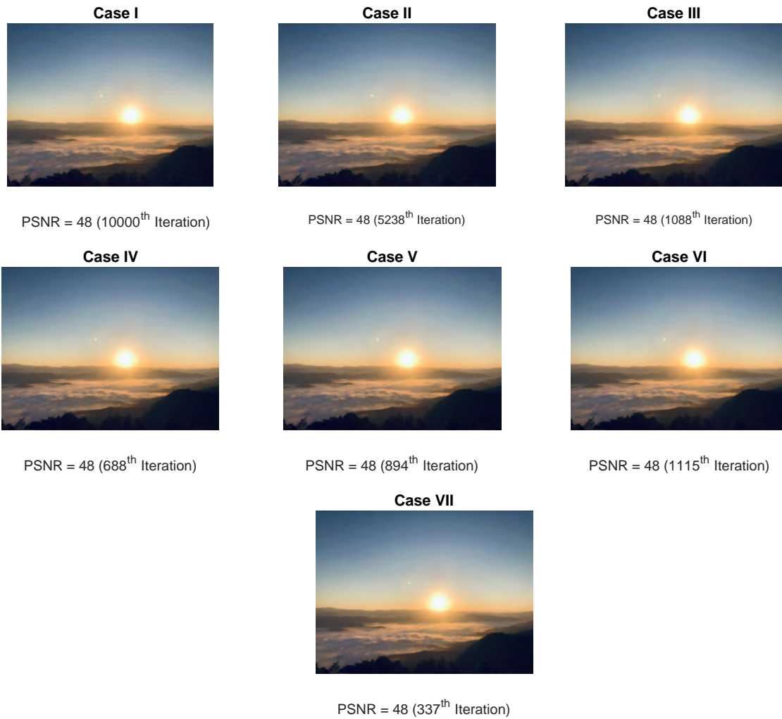
Figure 24-30: The reconstructed RGB images of all cases being used our Algorithm 3.1 with PSNR = 48.
