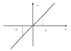
Figure 2: hard threshold function
