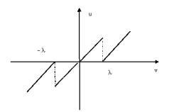
Figure 3: soft threshold function
