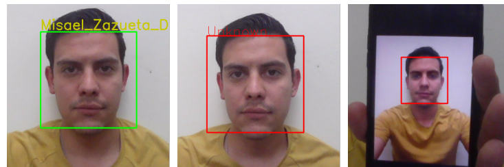
(a) Successful facial recognition in Screen. (b) Unsuccessful facial recognition in Screen. (c) Spoof try rejected in Screen.
