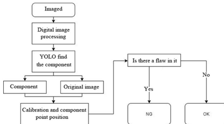
Fig. 3. Flow chart of the PCB inspection system
