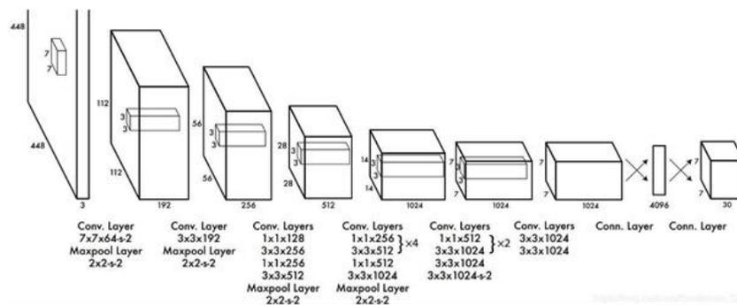
Fig. 2. YOLO network architecture diagram (Ki, 2017)
