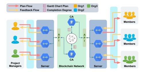
Fig. 3. Architecture of fabric-GC
