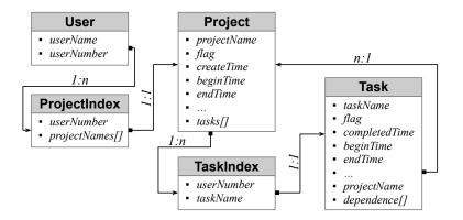
Fig. 4. Relationship between data structures
