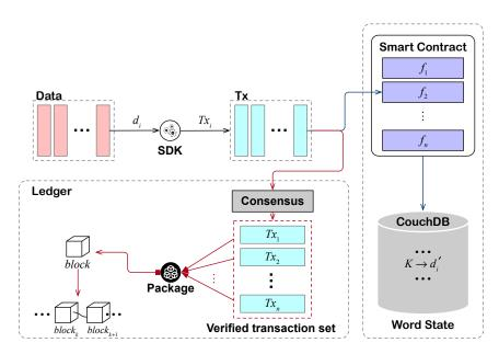
Fig. 1. Structure of the ledger in Hyperledger Fabric
