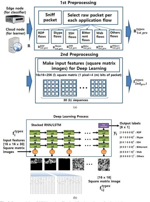
**Fig. 3.** Proposed deep RNN-based traffic classification scheme for the (a) data preprocessing and (b) deep learning process (Stacked RNN/LSTM)
