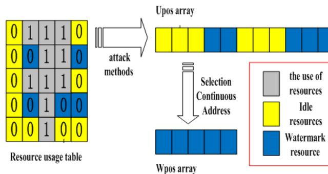
Fig. 2. Schematic diagram of the structure of the key generation
