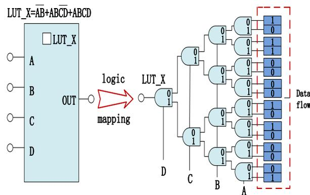
**Fig. 1.** The internal logical structure of LUT
