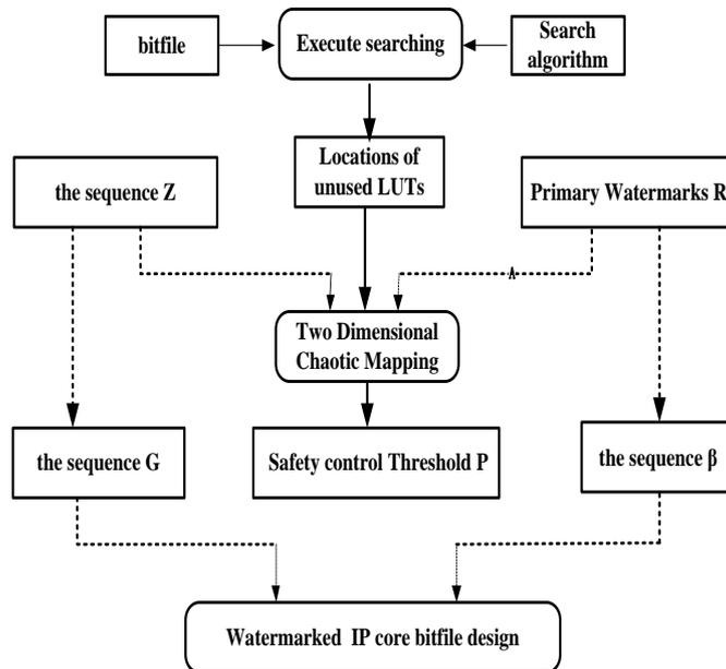
Fig.3. The flow of watermark embedding
