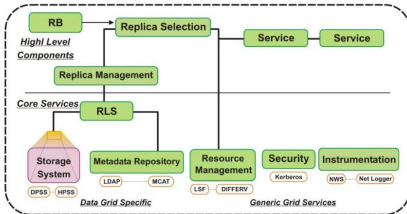
Fig. 1. Major components and structure of data grid architecture. (Adopted from[1])
