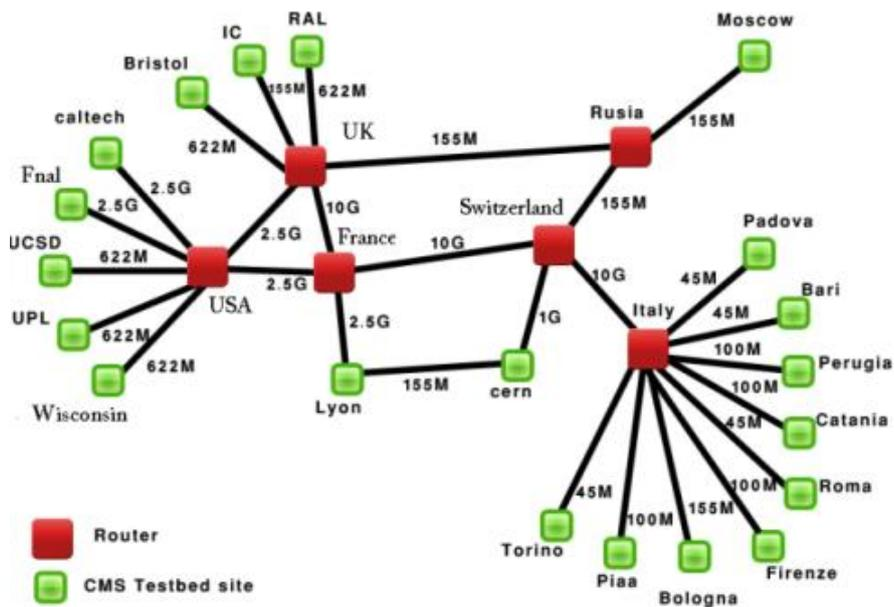
**Fig. 5.** Grid topology for CMS test bed
