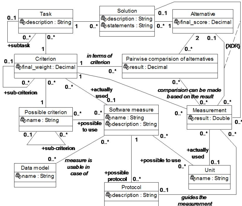
**Fig. 2.** A fragment of a metamodel of an evaluation method of database designs
