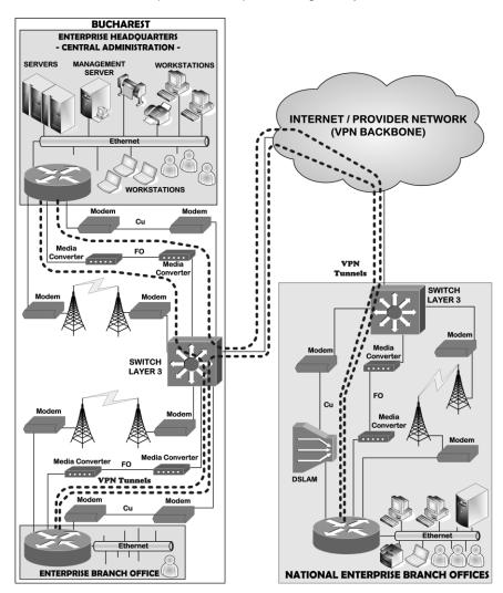
**Fig. 11.** A network general architecture with 3 loops (copper, fiber optic and radio), using the Internet or a provider network, for a large enterprise geographically dispersed to support transfer of large volumes of data over long distances
