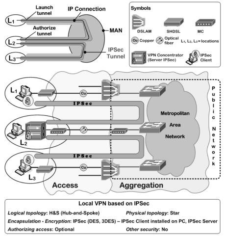
Fig. 13. Local VPN based on IPSec example
