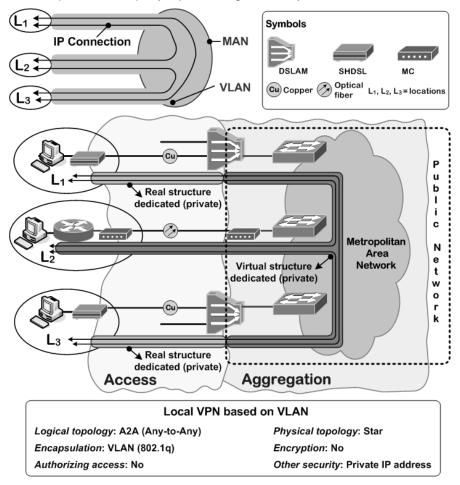
Fig. 12. Local VPN based on VLAN example
